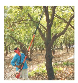
Ideal for cutting tree branches & foliage in orchards such as mango, apple, orange etc. From 6" to 8" diameter
