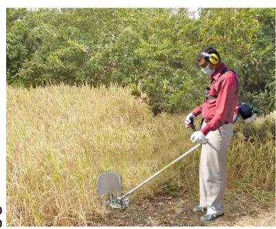
Suitable for harvesting paddy with paddy attachment. as well for cutting fresh or dry grass on ground, lawn, field etc.
